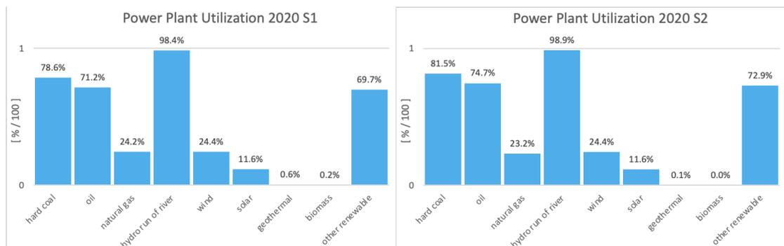
Figure 15: Left: detailed power plant utilization of Austria for Scenario 1; right: detailed power plant utilization of Austria for Scenario 2.
