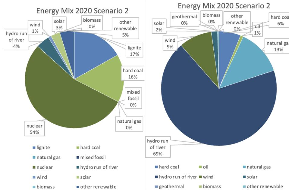
Figure 16: Left: Energy mix for scenario S2 2020 Czech Republic; right: Energy mix for scenario S2 2020 Austria.
