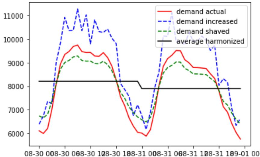
Figure 17: Demand shaving and increasing over 48 hours (harmonized average is the horizontal black line).
