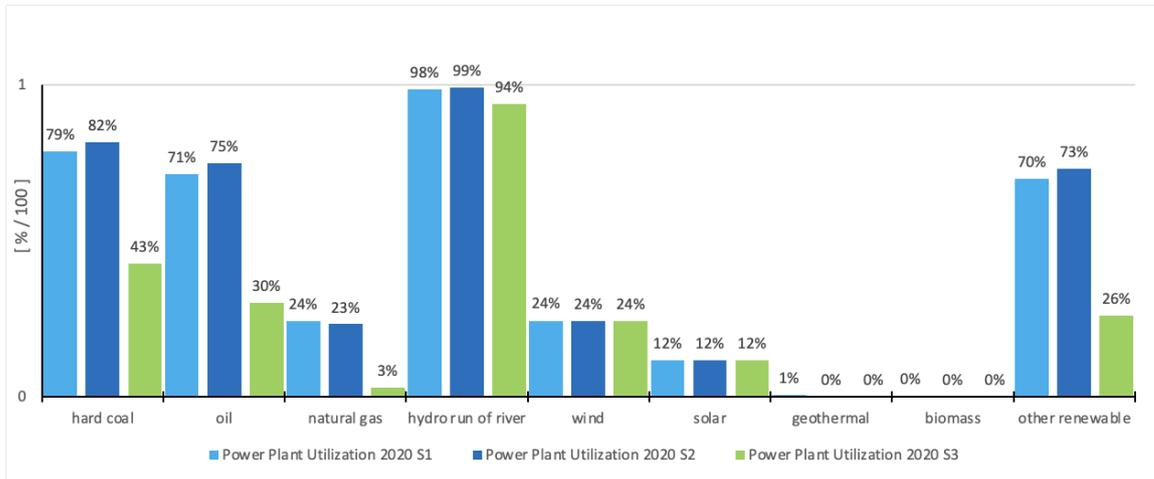
Figure 12: Power plant utilization for the scenarios S1 through S3 (predictions) for Austria, 2020.
