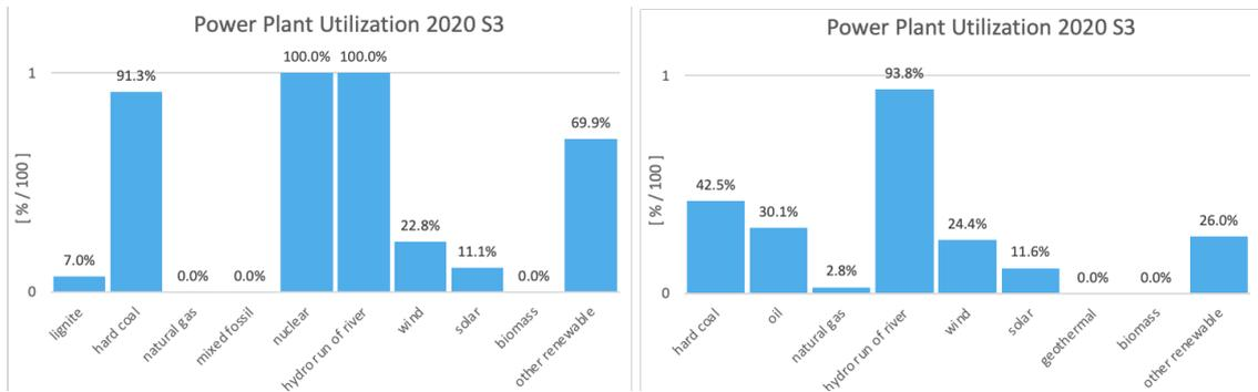
Figure 14: Left: detailed power plant utilization of the Czech Republic for Scenario 3; right: detailed power plant utilization of Austria for Scenario 3.
