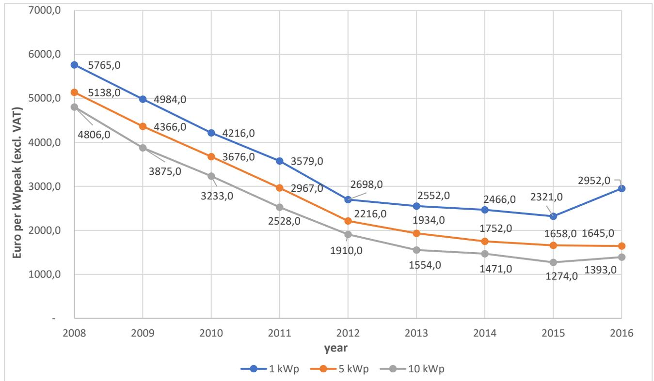
Figure 8 Specific system prices of 1 kWp-, 5 kWp- and 10kWp - PV-systems [6]
