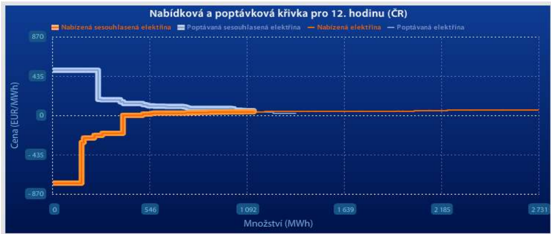
Figure 2: Matching curve in 4.3.2013. The white line is the demand and the orange line is the supply. Thick line is the realized supply. [Source: www.ote-cr.cz]
