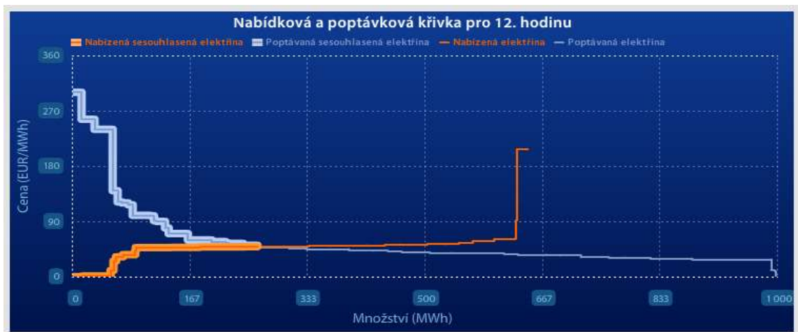
Figure 1: Matching curve in 9.3.2009. The white line is the demand and the orange line is the supply. Thick line is the realized supply. [Source: www.ote-cr.cz ]
